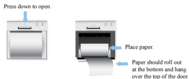
Printer paper installation (Fig.3-6)
